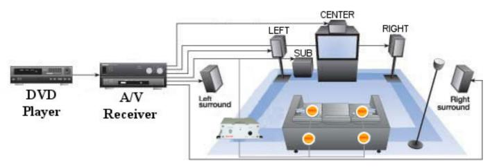
Our Vibrating Woofer Speaker is a whole new system adopting vibrating speakers under and back of the seats and linking AV receiver and vibrating amplifier to make user feel bass physically.
